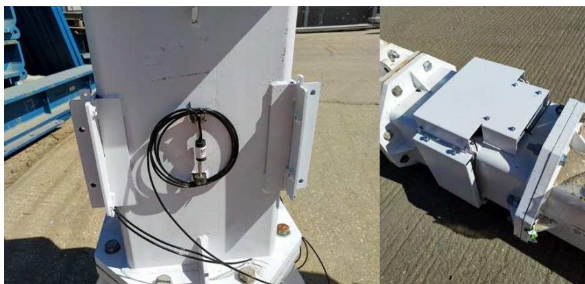
Figure 3: Load monitoring section showing strain gauges and protection to prevent damage.
