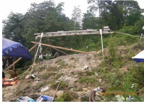
Figure 5: Artificial rainfall test in the field for validation of the MEMS tiltmeter technology (Sichuan Province, China).
