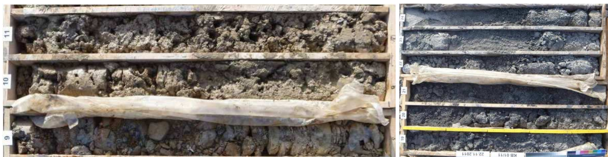
Figure 4: GA3 - Kakirite (KB 1/11, 18-24 m); GA4 - Greywacke schist, predominantly stratified, clearly deconsolidated (KB 2/11, 17-21m)
