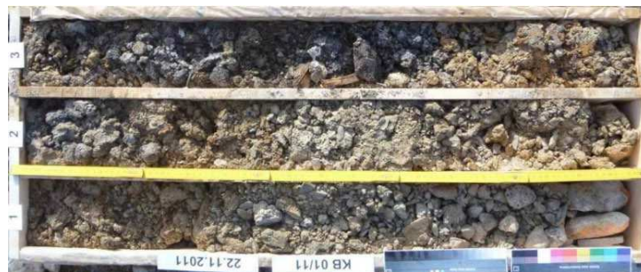
Figure 3: GA1 - Weathered material / slope rearrangement (KB 1/11, 0-3m); GA2 - Greywacke schist, predominantly deconsolidated (loose rock character) (KB 1/11, 8-11 m);
