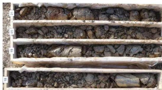
Figure 5: GA5 - Greywacke shale, in stratigraphy, dissected, weathered (KB 1/11, 29- 30,8m);
