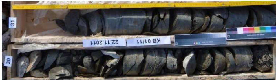
Figure 6: GA6 – Greywacke schist, stratified, un-weathered
