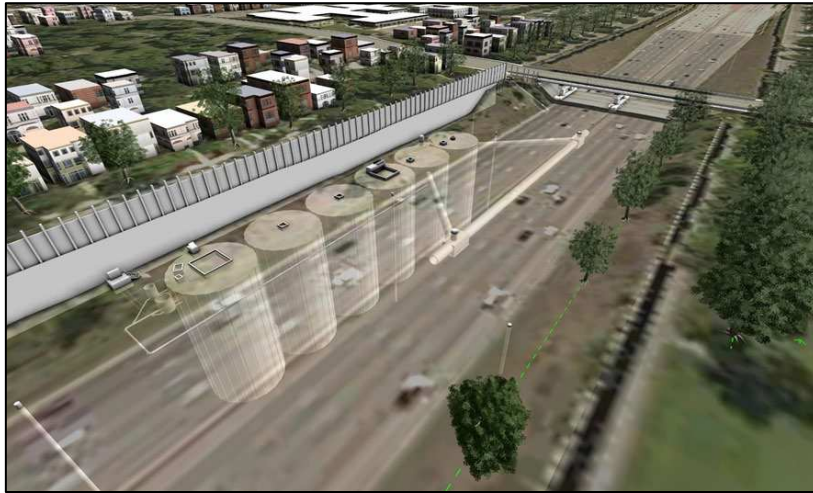
Figure 1: Concept design of the six cell Stormwater Storage Facility (SSF) – looking southeast
