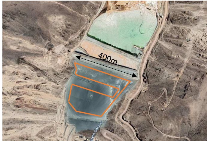
Figure 6: Deployment of about 2km of distributed strain sensing cable
