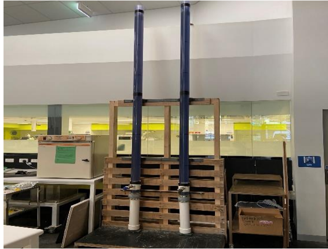
Figure 5: Two standpipe tube for test performance of MEMS piezometer
