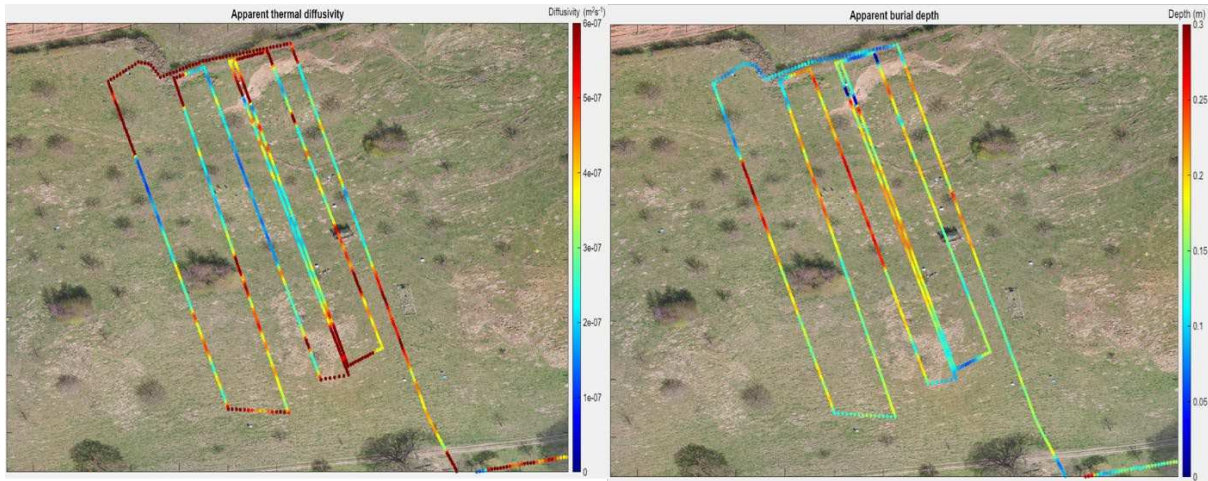
Figure 4: Left: calculated thermal diffusivity of the ground above the fibre mapped onto the slope, assuming a constant burial depth. Right: calculated burial depth of the fibre, assuming a constant thermal diffusivity.
