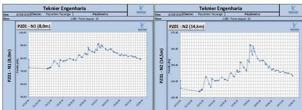
Figure 8: Monitoring piezometric data in PZ-01 at a depth of 8.0m and 14.5m.
