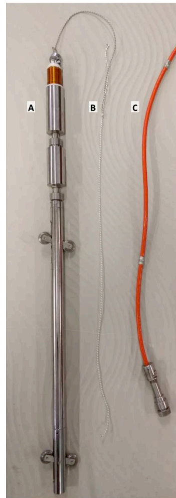
Figure 2. Incliner probe (A), Dyneema® cable, \phi 2.5mm (B) and traditional graduated cable, \phi 10 mm (C)
