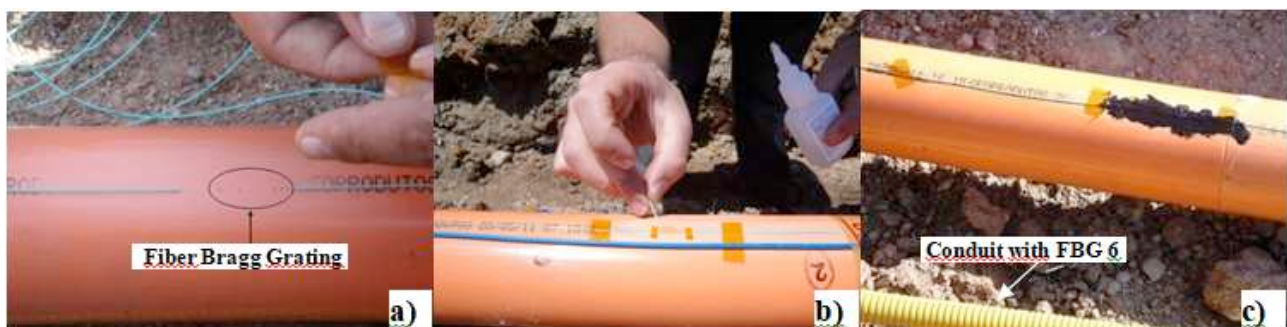
Figure 15. Fixation of FBG over the tube: a) clean tube; b) glue application; c) Adhesive sealant applied.
