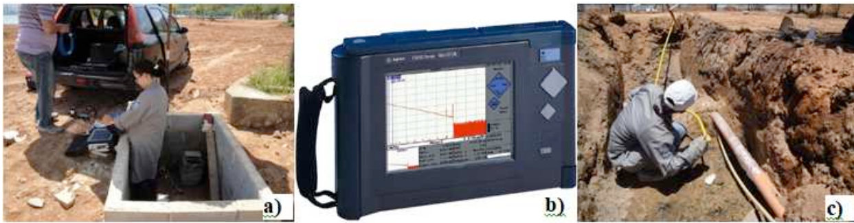
Figure 20. a) and b) Analysis of FBG transmission with OTDR; c) local of the splicing
