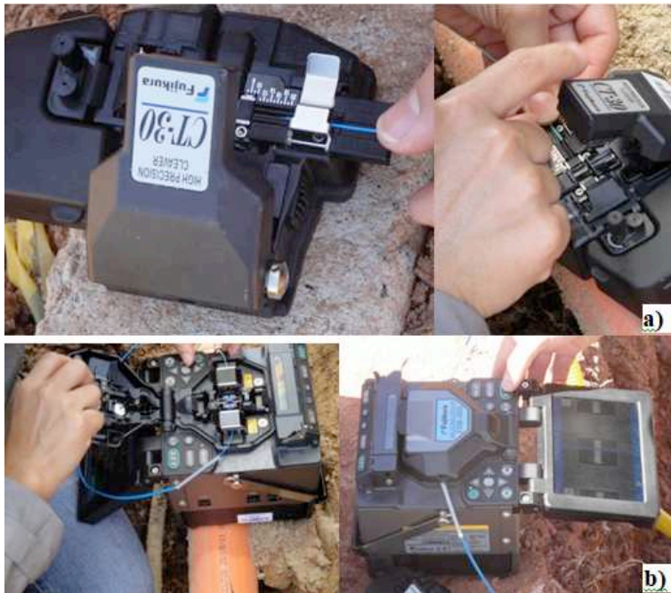
Figure 14. Cleavage and splicing of the FBG.
