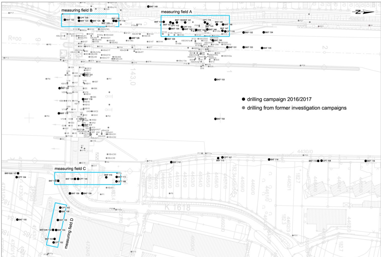
Figure 3. Ground plan of the site with measuring fields for geophysical investigation, marked with a turquoise frame.
