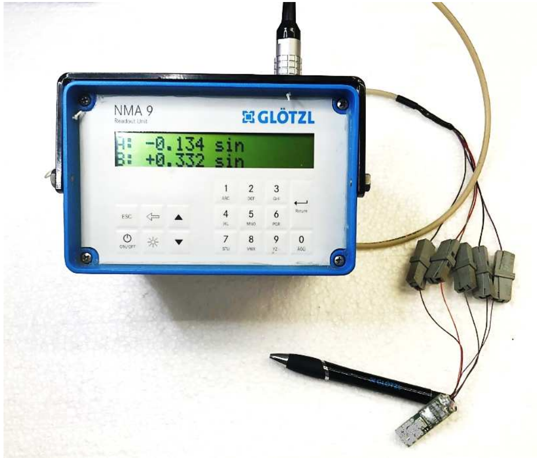
Fig. 14- Glötzl hand-held readout unit for inclination sensors connected to the MEMS
