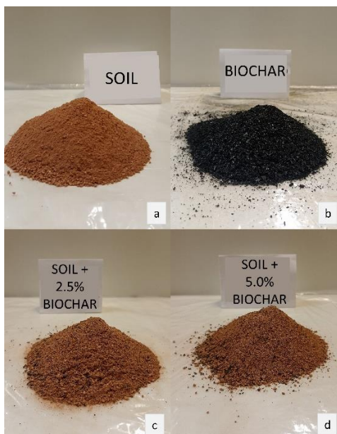
Figure 1. Soil sample (a), pruning waste biochar (b), mixture of soil with 2.5% biochar (c), and mixture of soil with 5% biochar (d).
