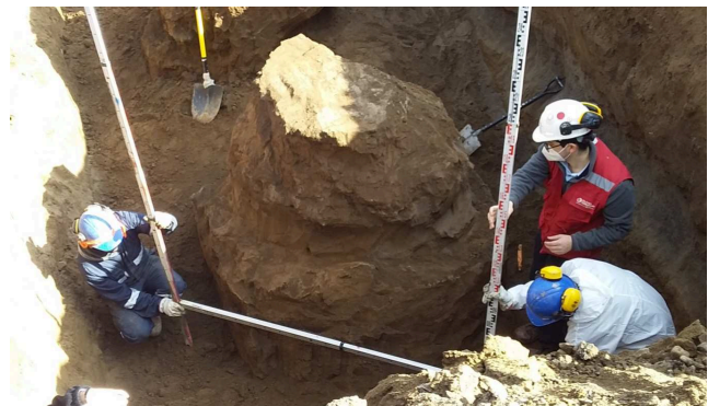
Figure 6. Exhumation of Jet Grouting Column in silts, Northern Santiago (ref. Pilotes Terratest).
