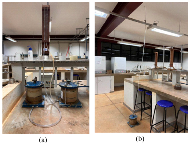
Figure 5: Sample saturation on the variable head apparatus: (a) SG sample; (b) LR sample saturation using a high elevation head approach.
