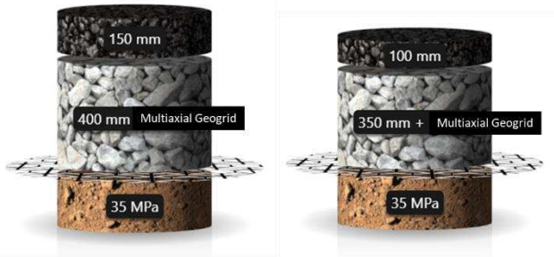
Figure 2. Alternative Pavement Sections Using an MSL
