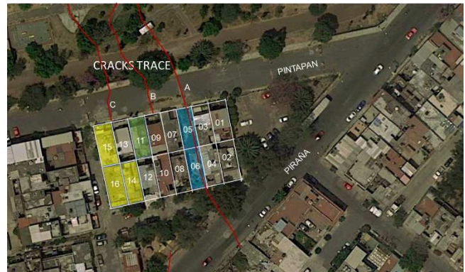
a) Plant, cracks path on the surface of the ground. Modified from Google Earth (2017).
