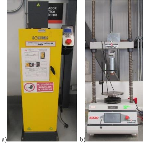
Figure 7. Equipment used for CBR testing.
