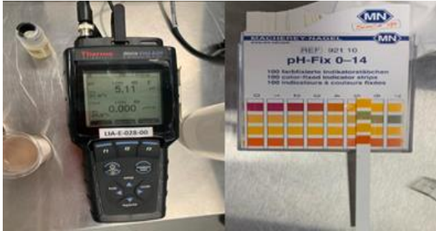
Figure 4. Determination of pH: Quantitative and qualitative Analysis
