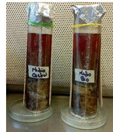
Figure 2. Experimental setup number two and three using acetate sheets for bio-sealing fractures in rock using addition and change of media as different assemblies.
