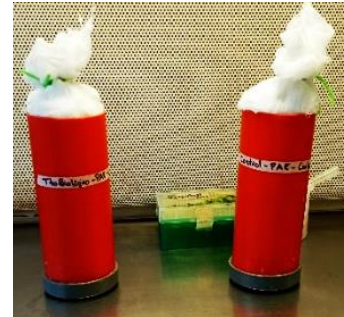
Figure 1. Experimental setup number one using PVC tubes for bio-sealing fractures in rock.
