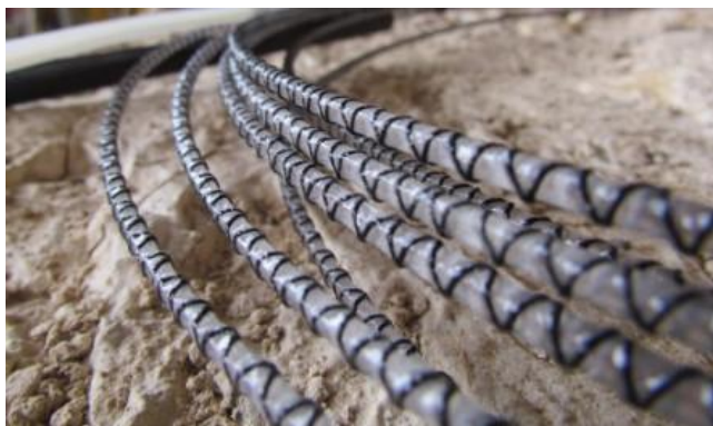
Figura 2. Cable DFOS ODISi/ Nerve .
