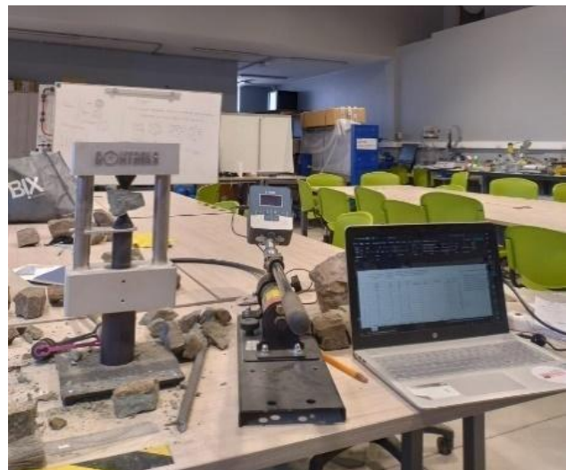
Figure 3. The point load strength tests in the Geomechanics laboratory of Universidad de O'Higgins.
