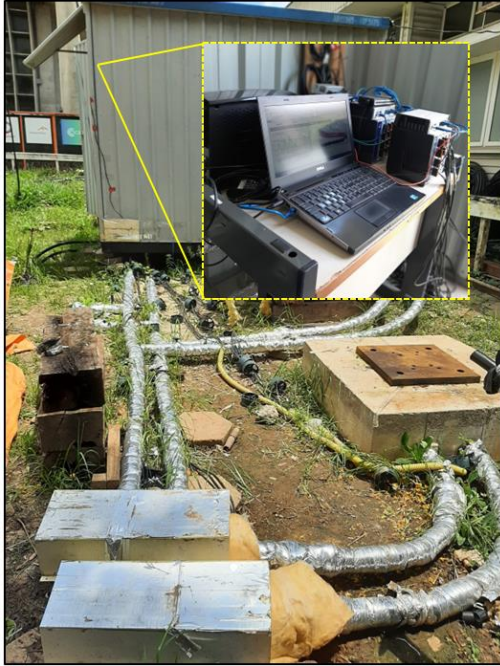
Figure 4. Overview of the system, showing the insulated pipes, the container, and a detail of the data acquisition system.
