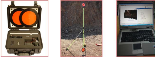
Figure 1. System components. Calibrated camera (left); Range pole (center); software (right).
