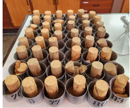
Figure 11. Photos of dried oven samples after the UCS testing
