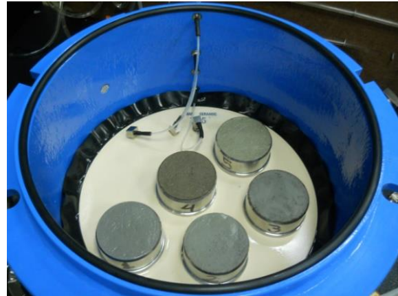
Figure 4. Samples in SWCC test with pressure extractor plate.
