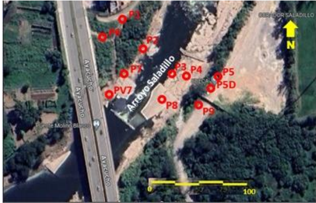
Figure 8. Location of geotechnical borings.
