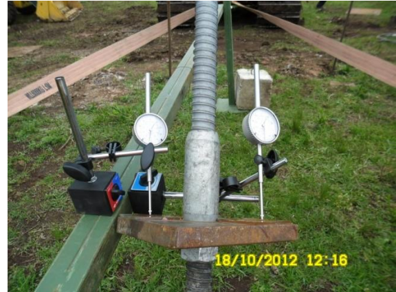
Figure 2. Strain measurement system for brace testing – Site 1.
