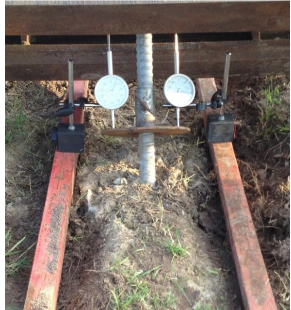
Figure 8. Breakage of soil surrounding the grout. Location 283 - Site 2.
