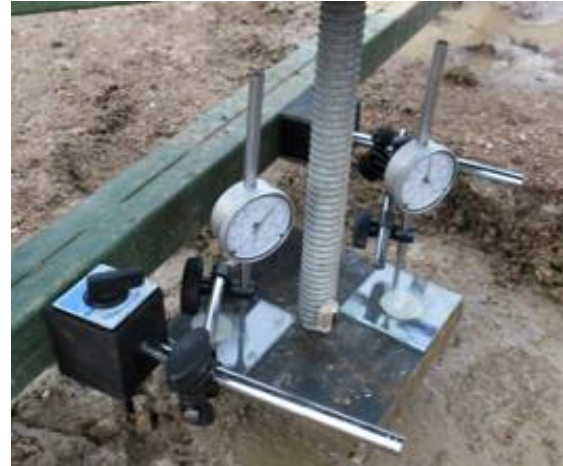
Figure 5. Strain measurement system for vertical anchors - Site 1.
