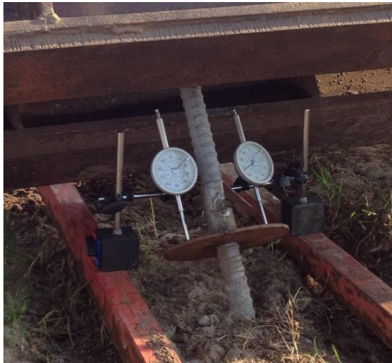
Figure 7. Strain measurement system for inclined anchor testing - Site 2.
