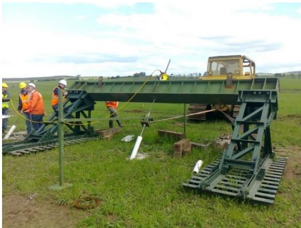
Figure 1. Reaction system for brace testing – Site 1.
