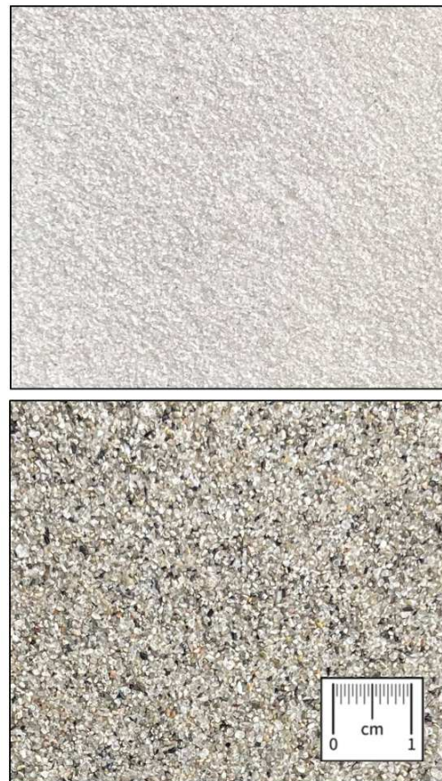
Figure 1. Fine-medium Ottawa (upper) and Guamo (below) sands particles under study, based on the Unified Facilities Criteria (U.S. Army Corps of Engineers, 2022).
