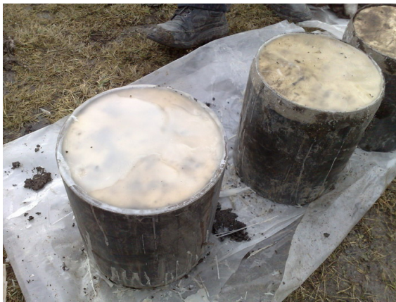
Figure 2. Waxed peat samples inside the samplers
