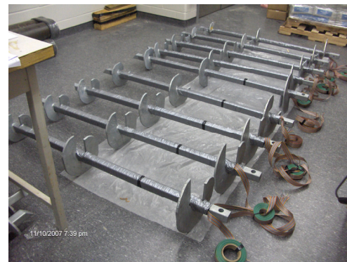
Figure 4.b. Finished instrumented lead sections
