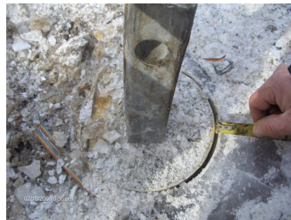
Figure.13. FRP-G-HSP with external grout separation between the FRP tube & external grout during lateral testing
