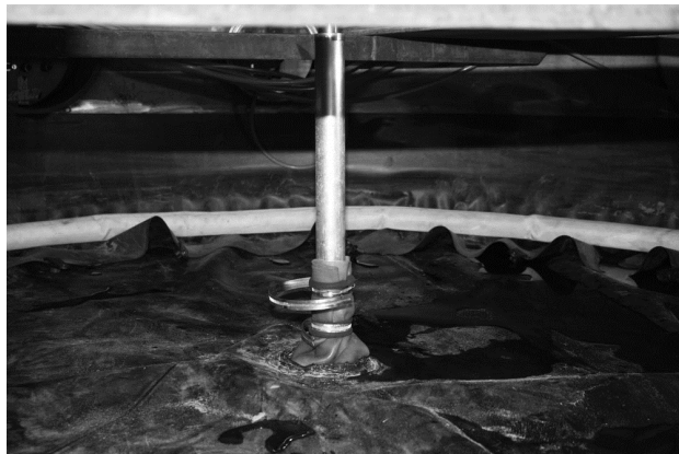
Figure 4. The membrane placed on the soil surface and secured around the pile by hose clips and against the side of the tank by a fire hose.
