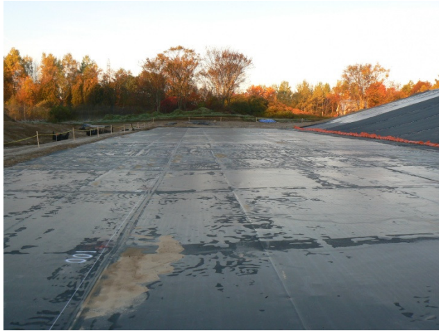
Figure 6 Photo of a GM in direct contact with the underlying GCL liner at QUELTS at 7:00 am on a cool October morning. Note left-right width of base to the orange sand bags at toe of slope is about 20 m.
