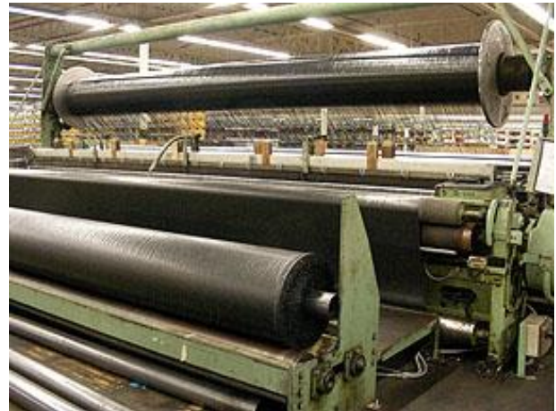
Figure 4. High strength woven geotextile loom that can make geotextiles with stacked tapes.
