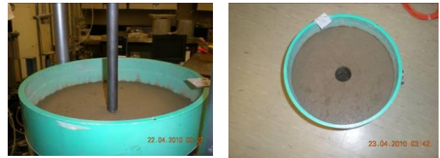
Figure 4. Driving a hole in the compacted soil using thin-wall steel tube for installing the model pile.
