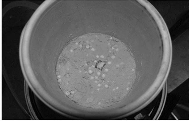
Figure 4. Clay specimens for cyclic triaxial test: mixed specimens containing 40% (volumetric) Ceramic beads
