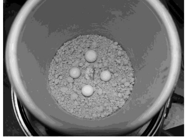
Figure 5. Clay specimens for cyclic triaxial test: pure specimens, with inclusions around the IPT
