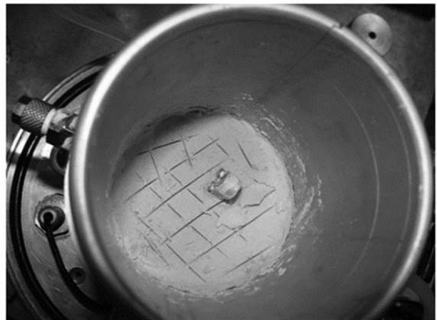
Figure 2. Clay specimens for cyclic triaxial test: pure clay specimen with the IPT (inclusion-free) inside
