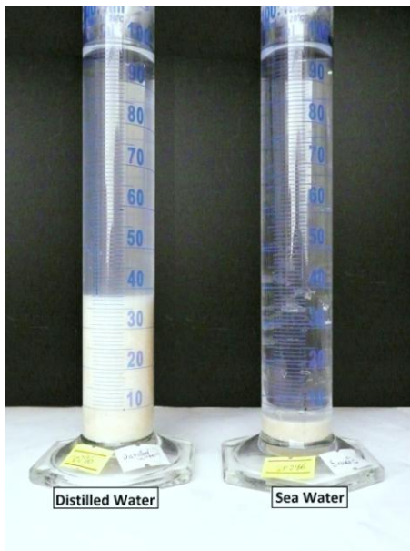
Figure 3. Modified free swell index (MFSI) determination of the samples
