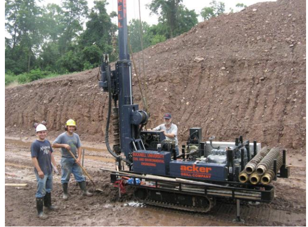
Figure 2 Drilling rig used for cutoff wall testing
