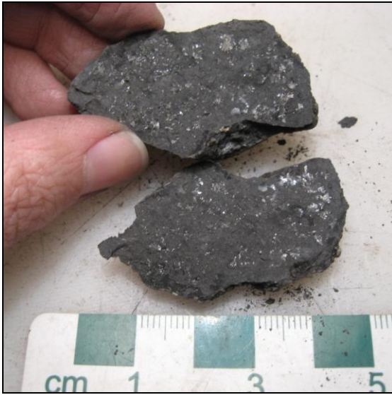
Figure 2. Visible gypsum crystal clusters on faces of freshly opened lamination
