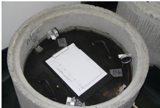
Figure 4. Monitoring gauges in place at start of test
