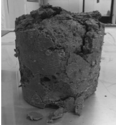
Figure 2- Degradation of a specimen after 7 f/t cycles
