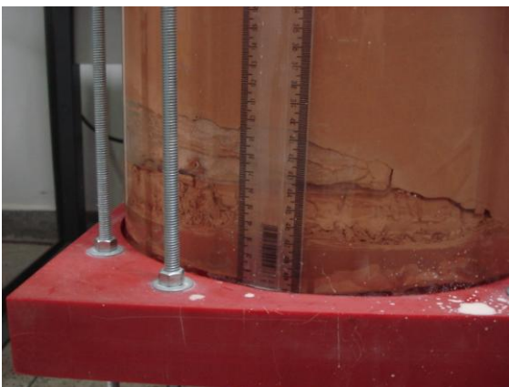
Figure 9. Shrinkage at the bottom of model after reversal of polarity
