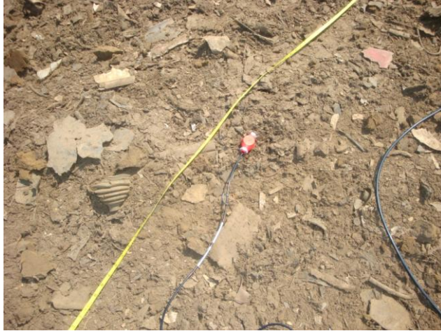
Figure 12. View of auto shredder residue (auto fluff) with geophone for scale
