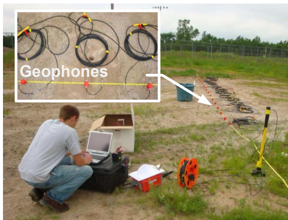
Figure 2. View of MASW test in a landfill in Michigan
