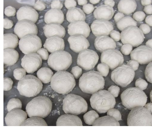
Figure 6. Clay balls made for simulating lumpy soil
