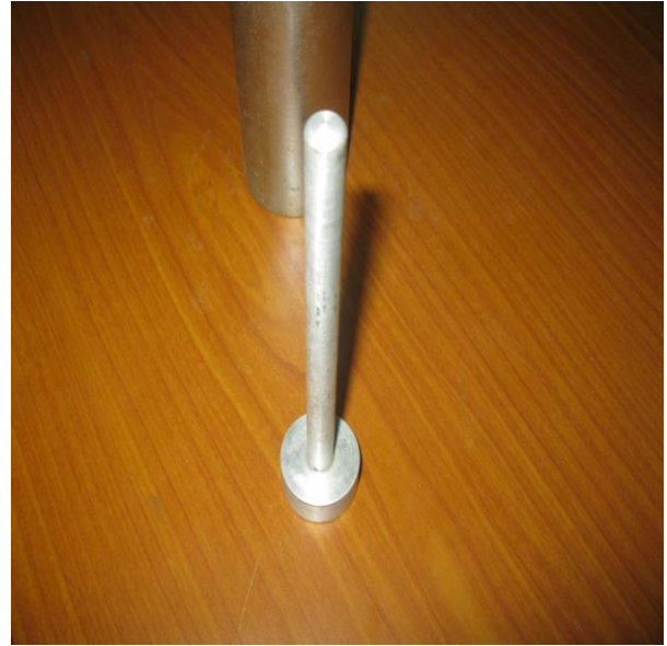
Figure 3.(b) Hammer used in Wet tamping
