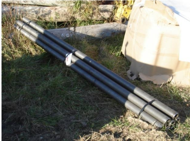
Figure 2. B7X1-76 Geo-drilled hollow core injection bars
