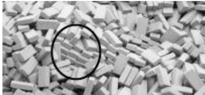
Figure 7 Evidence of the initial structure in a final deposit of a test of 40,000 cm 3 of piled bricks with a smooth slope break (Manzella and Labiouse, 2011)
