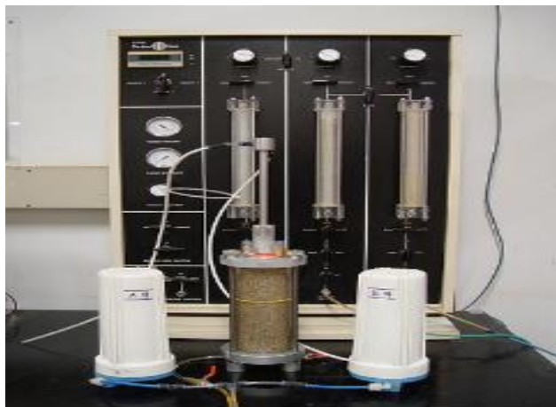
Figure 1. Sandgel compressive strength test
