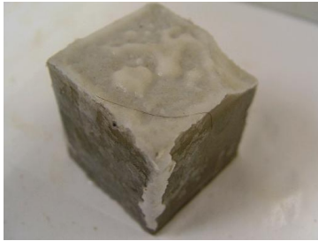
Figure 9. White precipitate from homogel under sea water
