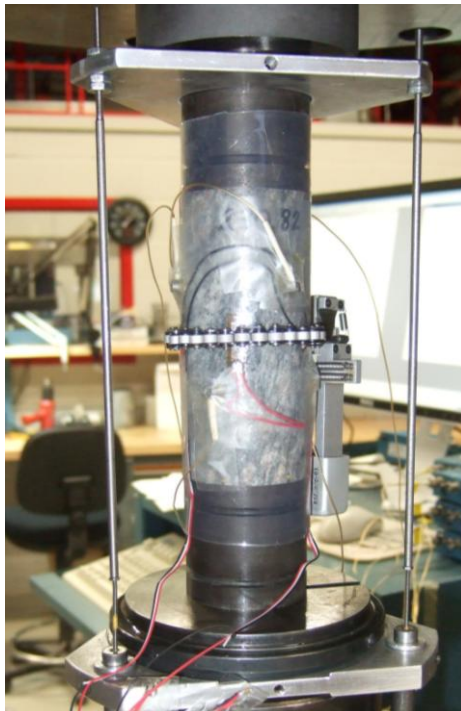
Figure 10. A Smaland granite specimen ready for testing, the specimen was monitored by AE sensors, vertical and horizontal strain gauges, LVDTs for axial deformation and extensometer for circumferential strain (Courtesy of ISRM Commission on Spalling Prediction).
