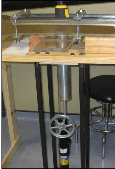
Figure 1. Extrusion and Erosion Measurement System
