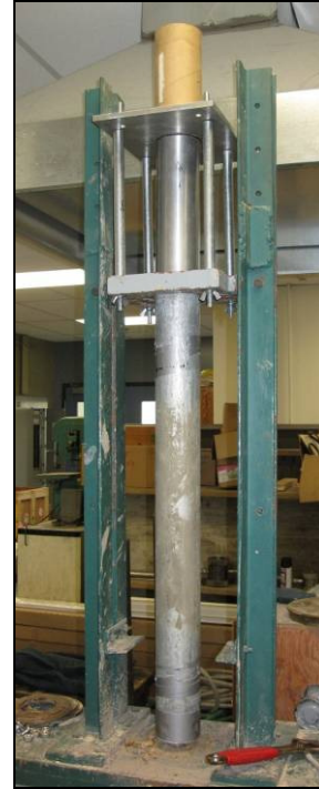
Figure 2. Extraction of Sample from Shelby Tube into the tube fitted for the EMD
