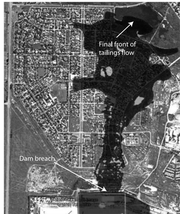
Figure 5. The result of Merriespruit tailings dam failure simulation superimposed on satellite imagery (Google Earth 2010)
