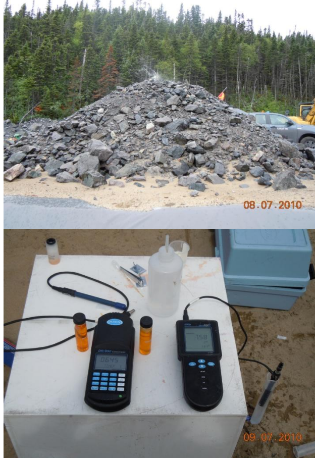
Figure 4: Field set-up for retention tests: water sprinkler on top of cell (top) and colorimetry and pH/ORP equipment (bottom).
